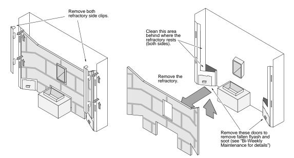
Clean the Exhaust Duct (make sure the heater is cool and unplugged)
